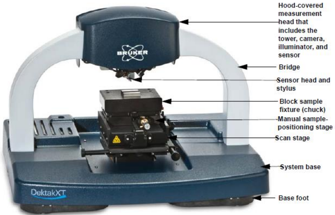
Figure 1 DektakXT Stylus Profiler equipped with manual X-Y stage
