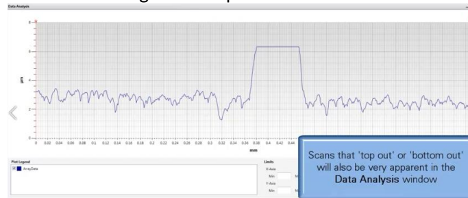
Figure 7 Scan Range with inappropriate scan range / scan profile setting.
