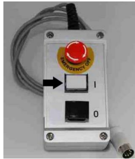
Figure 3 Emergency Machine Off (EMO) Box
