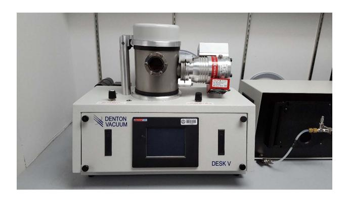
This tool is designed to provide a thin conductive coating of a few monolayers on nonconductive samples to allow analysis in a SEM. The system is not designed to deposit thick layers for materials research and should not be used for thick layers.
