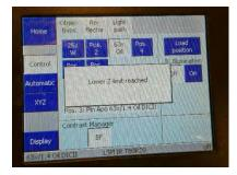
control panel it shows Lower Z-limit reached. If this does not show up, turn the knob (down direction) to show it up. Then click 'calibrate'.
