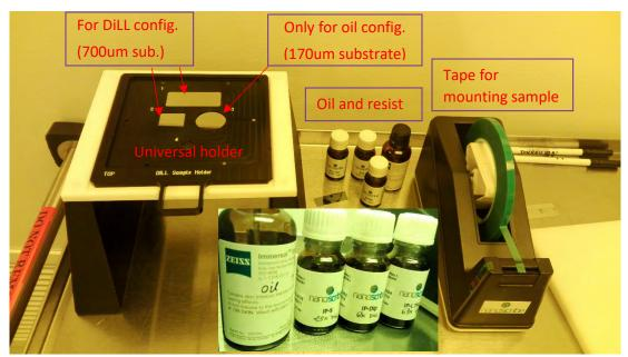
Dill config.: Put the holder bottom up, mount the substrate onto the predefined position with the tape. Then dip a droplet of resist to the center of the substrate. Oil config.: Put the holder bottom up, mount the substrate onto the predefined position with the tape. Then dip a droplet of oil to the center of the substrate. Flip the holder and dip a droplet of resist to the backside center of the substrate.
